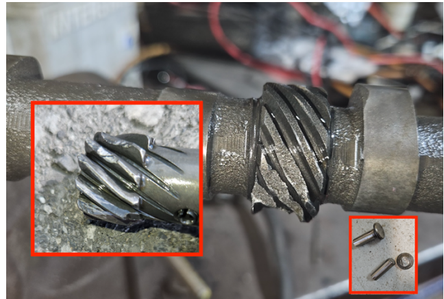
Camshaft and distributor gears, eaten. Broken lifter.
